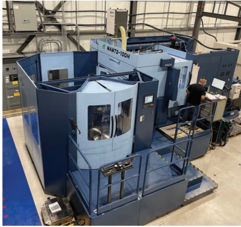
The company has planned a complete upgrade of its CNC machines and has started with a Matsuura MAM72-100H 5-axis machining centre, a Matsuura MAM72-70H 5-axis machining centre, and a Nakamura-Tome JX-250 turn-mill centre.
